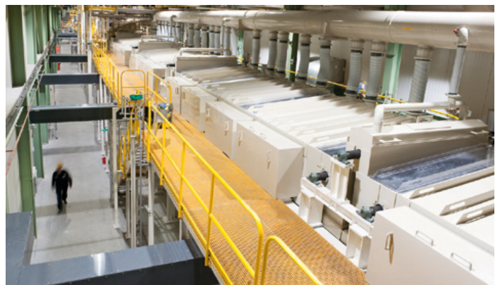
Anodising is the third stage of the micro-graining process
