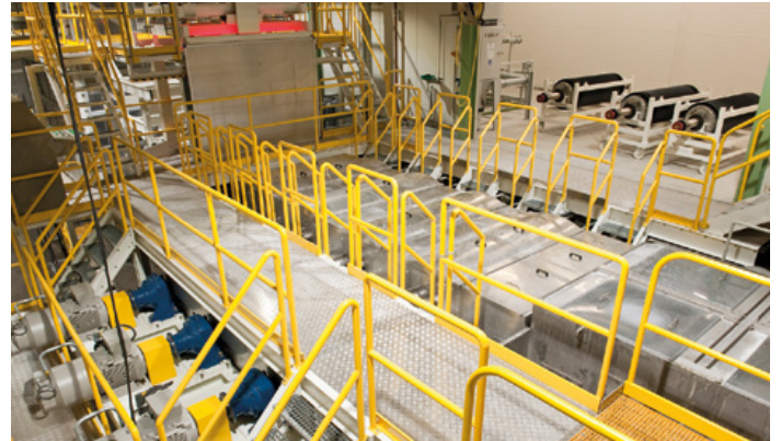
Brush-graining is the first stage of the micro-graining process
