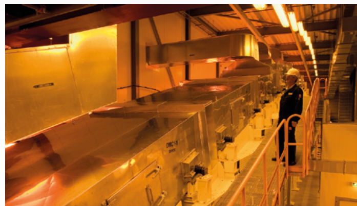
The coated layers are dried prior to automated laser inspection
