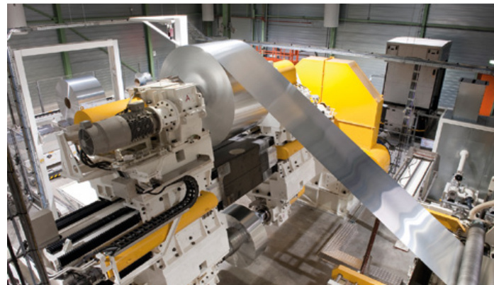
Unwinding and joining process ensures consistent 24/7 operation
